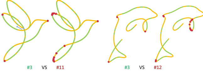
Fig. 2. Comparison of the number of tuned points of our beam search method (left figure of each model) and the greedy-based method (right figure of each model). Our method can obviously reduce the manual operation cost. Our algorithm takes 22.11 seconds on average, and the greedy-based method takes 13.57 seconds on average.
