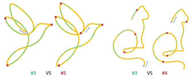
Fig. 5. Illustration of reversing the sequence of wire. After the fitting is completed, we reverse the fitted elements sequences, getting different number of tuned points. We select less one for final fabrication.
