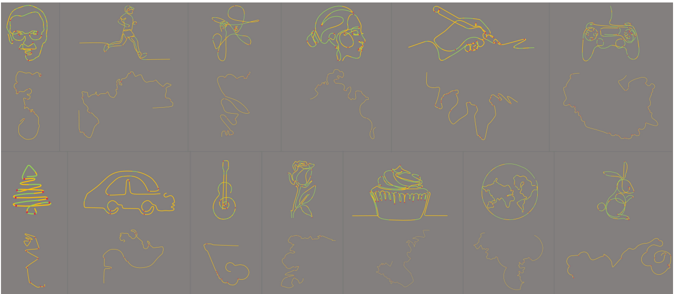
Fig. 8. Thirteen results of 2d wire art examples. The models are arranged in the order of Man , Runner , Hat woman , Side face woman , Writing , Game player , Tree , Car , Guitar , Flower , Cake , World map , Rabbit . We show both the fitting result (line segment: Green, circular segment: Yellow) and the tuned wire.
